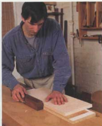
Shoot the edges. A stroke or two with a jointer plane prepares the veneers to be joined edge to edge.
