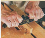
Cut the beading. For a smooth cut with a beading tool, take light passes across the edge of the board.
