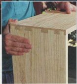
The variable-spaced, half-blind dovetail joint is complete. Templates can be custom-made for any project of any width.
