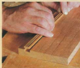
Set the beading in place. The beaded stock is glued into a groove ripped on the drawer front.
