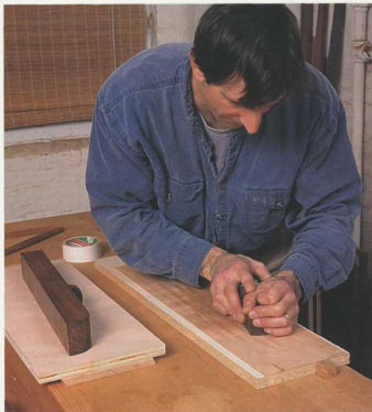
Smoothing after sawing. Double-stick tape keeps a sheet of veneer still for a quick smoothing with handplanes. At \frac{1}{8} in. thick, the veneer can be planed and worked like solid wood.
