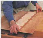
Taping under way. Short pieces of veneer tape are moistened and stretched across the joint; when they dry, they pull the joint tight. A lengthwise strip of tape reinforces the temporary joint.
